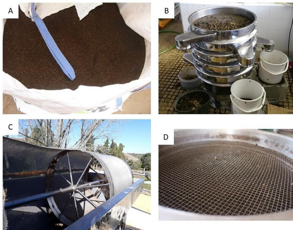
Figure 13 - Substrate converted into organic fertilizer and the separation process. A - converted substrate/organic fertilizer, B - semi-industrial vibratory sieve, C - rotational drum sieve, D - detail of vibratory sieve. (EntoGreen images)
