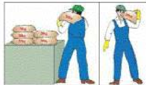
Figure 16. It is always better to use smaller packages. Loading and unloading may require more trips, but fatigue will be reduced.
