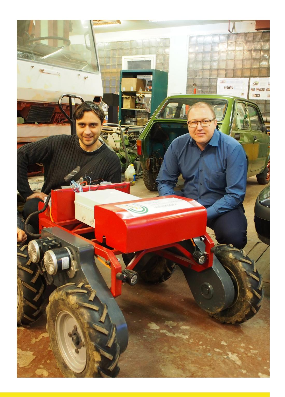
Within the project it is planned to develop a weed management equipment that would be able to autonomously move on a field and identify weeds and crops, as well as a high-power laser or precisely positioned mechanical tool is going to be used, to destroy the weed or considerably hinder its further growth.
